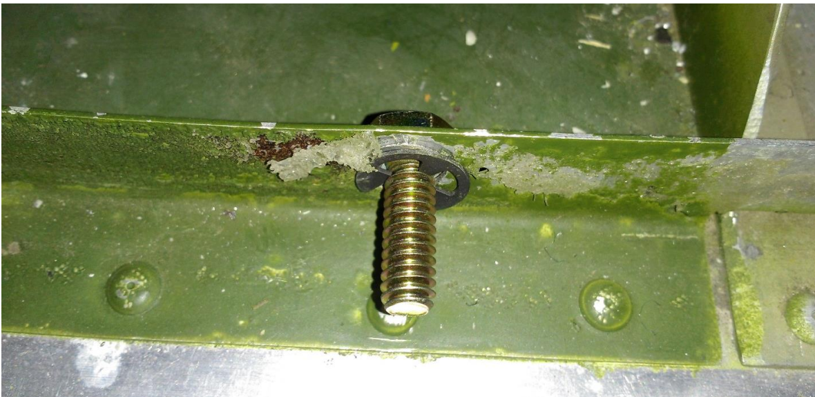
Figure 10. Lower mounting bolt as installed with the e-clip retaining ring. There is a washer on the back side of this assembly (not visible).
