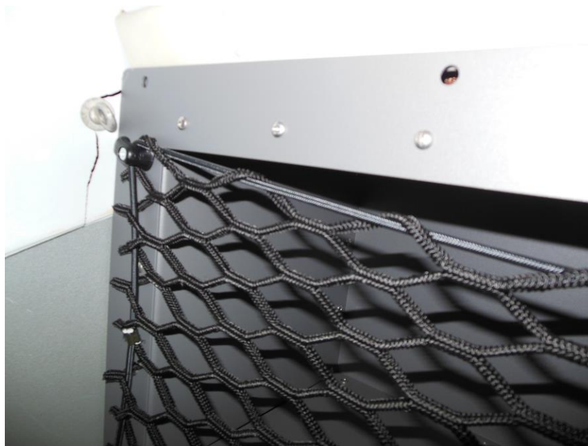
Figure 12. Pointing out the eyelets that may interfere with a smooth installation.
