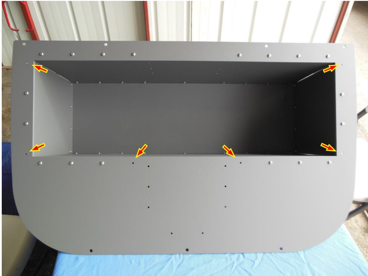
Figure 5. Bulkhead as installed with six holes unfilled.
