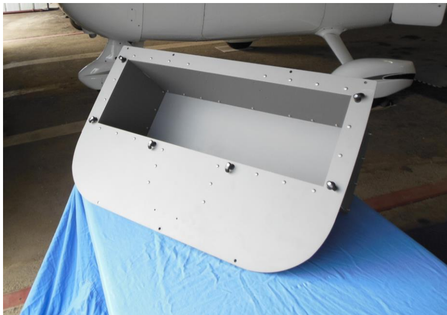
Figure 8. Aft Bulkhead Assembly with net hooks installed.
